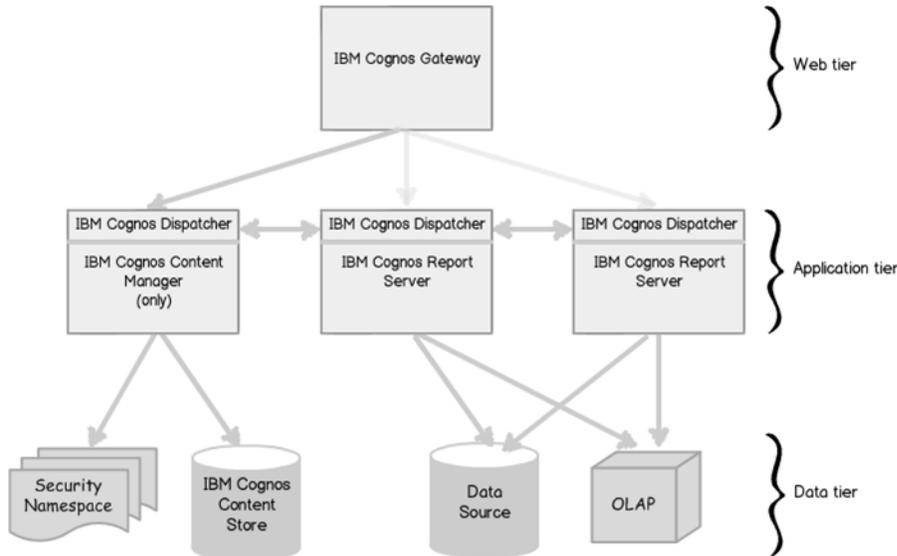
**Figure 1: An example of an IBM Cognos deployment**
