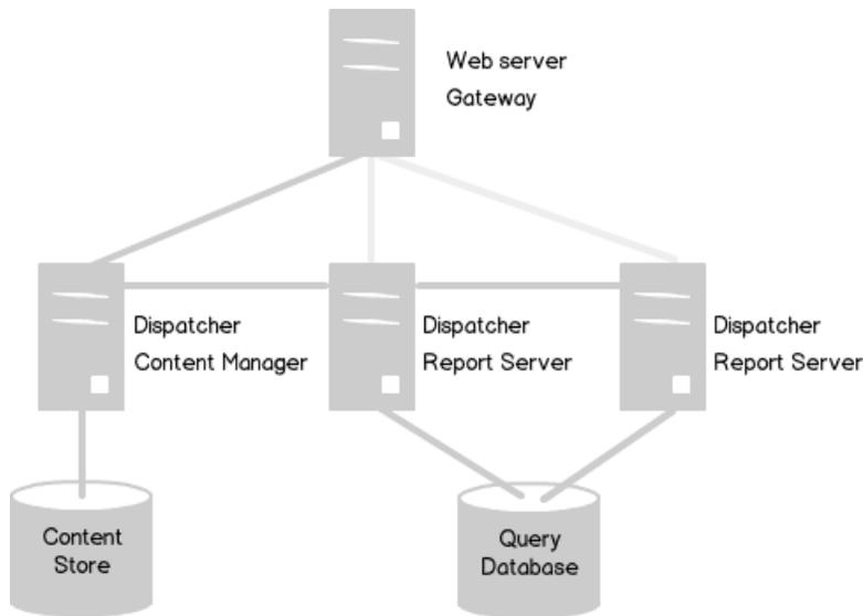
**Figure 5: More than one Application Tier components computer**
